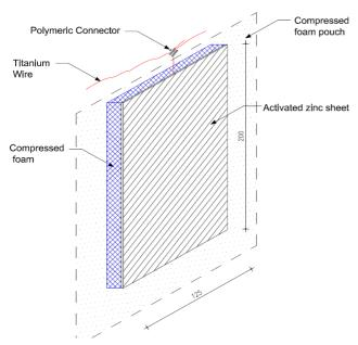
Compressed foam is 3x thicker on large anode variant
