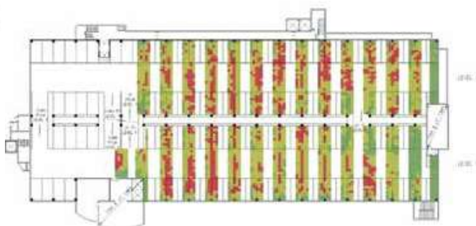
Figure 9: Pre-Installation Steel Potential Survey with ASTM C876 Colour Coded Corrosion Risk Bands.
