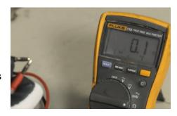
To obtain the required resistivity it may be necessary to use metal tie wires to connect the reinforcing bar to achieve electrical continuity.
