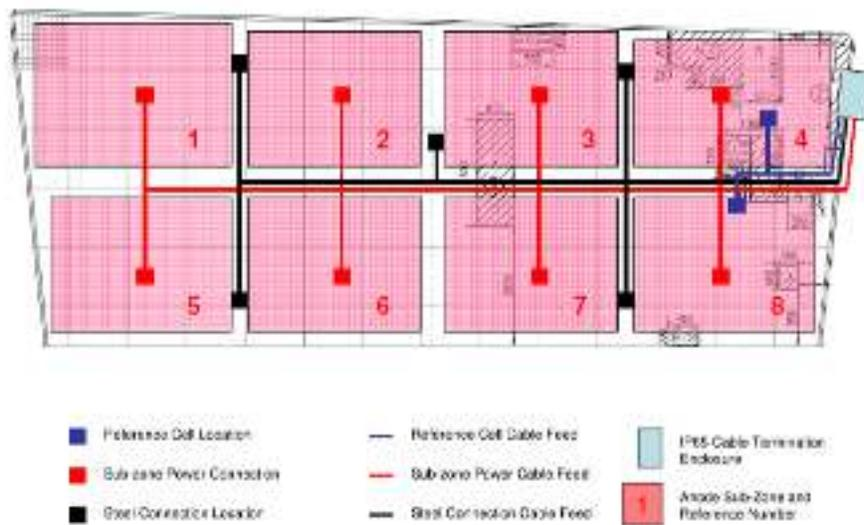
Figure 29 - Arrangement of hybrid anode zones, steel connections and reference cell locations
