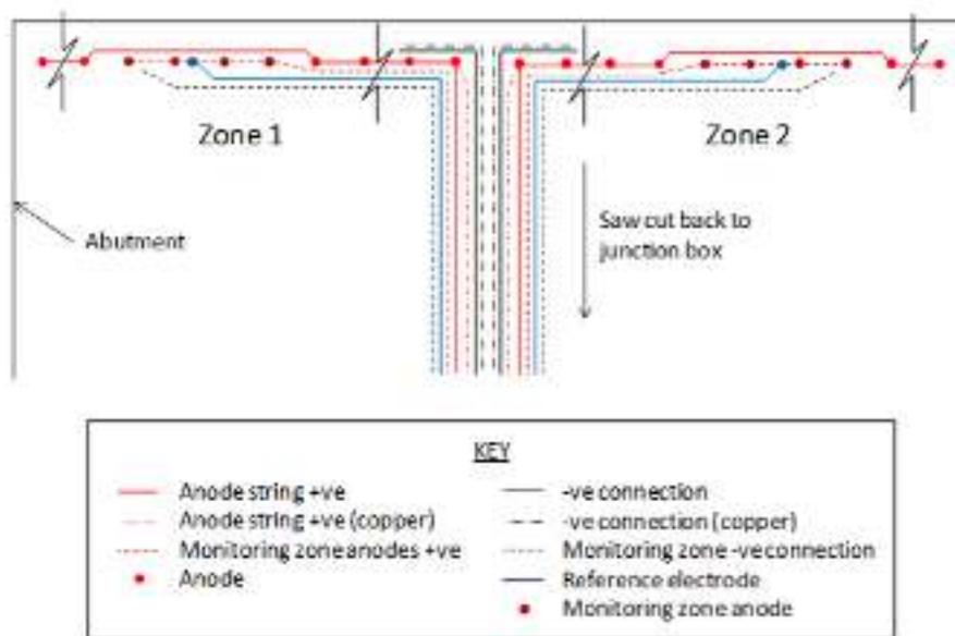
Figure 39 - Wiring schematic for M69 abutments Hybrid anode installation
