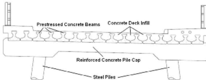
Figure 3 - Typical cross section of bridge deck
