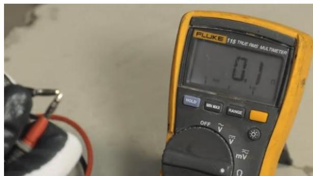
Confirm steel reinforcement continuity in areas to be treated by checking a sample of bars within the patch.
